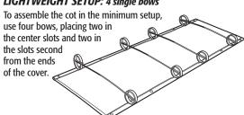
**Tip:** You can place single or twist bows in different slots to create a setup with custom support.
